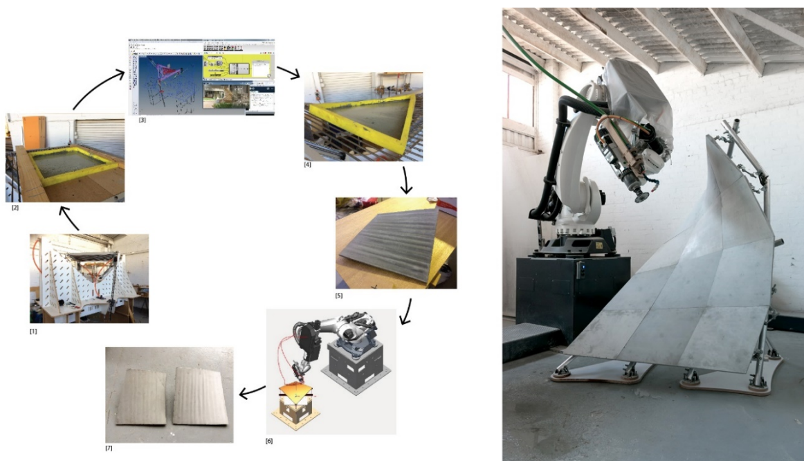
Figure 5. PAM technology and its fabrication procedure for the doubly curved concrete panel using a single adjustable mould. A full-scale rainscreen façade prototype was constructed as proof of concept to commercialise the technology.
