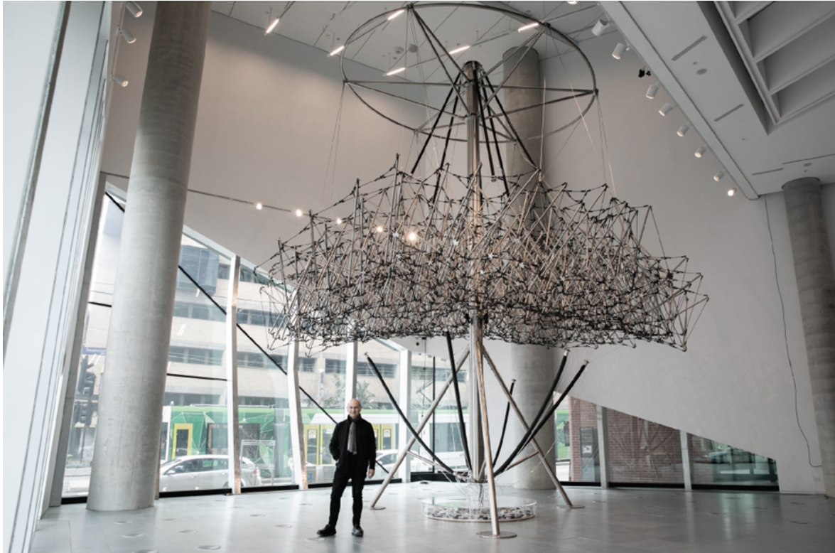
Figure 7. The Anthropomorphic Machine installation in Science Gallery Melbourne with an actuated suspended tensegrity "cloud" actuated by 12 pneumatic rubber muscles.
